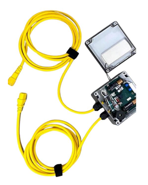
The Flair Model SZA460 can be used to combat theft and secure your property. Two heavy duty cables run through the equipment and plug in to each other to form a loop. If the loop is broken or cut an alarm is triggered. The annunciator has a large magnet on the back of the case so that it will securely attach to the equipment it is protecting. Adding an Inovonics EN1210 wireless transmitter will allow you to trigger an alarm at remote location for immediate attention.
