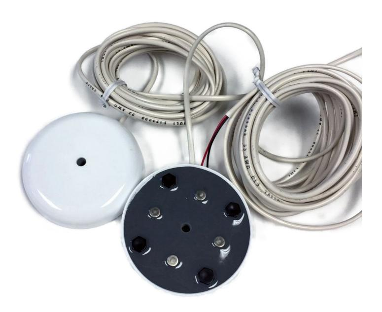
The Flair Model 3010-H2O-EN1751 Waterguard Probe connects to the Inovonics EN1751 Transmitter and are designed to detect water or any electrically conductive fluid. These sensors are mounted under water heaters, behind dishwashers, under sinks or on the floor of sensitive areas like computer rooms. If there should be a leak, the Waterguard Probe will sense it and trigger a wireless alarm immediately.
