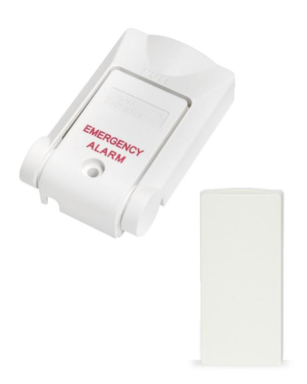
The Flair Model FLR-3045 low-profile panic switch can be mounted on the wall or under a desk out of sight and will not snag on clothing. Pulling the lever activates the switch and triggers a call. The smooth operation and noticeable click of the lever let's the user know that the switch is working properly. Adding an Inovonics EN1210 wireless transmitter will allow you to trigger an alarm at remote location for immediate attention.
