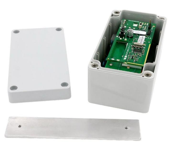
The Flair Model VIB450W Wireless chain link and metal bar fence Vibration Sensors catch the bad guys before they can get into your facility. These stand-alone sensors attach to the fence with just two screws. An onboard microcontroller analyzes the vibration at the fence and makes the call - Is it a person attempting to climb or cut the fence or just a little breeze? Select from multiple sensitivity profiles to reduce false alarms and optimize settings to the type of fence and intrusion.
