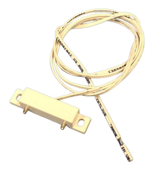
The Flair Model 1010-H2O-EN1751 Waterguard Probe connects to the Inovonics EN1751 Transmitter and are designed to detect water or any electrically conductive fluid. These sensors are mounted under water heaters, behind dishwashers, under sinks or on the floor of sensitive areas like computer rooms. If there should be a leak, the Waterguard Probe will sense it and trigger a wireless alarm immediately .
